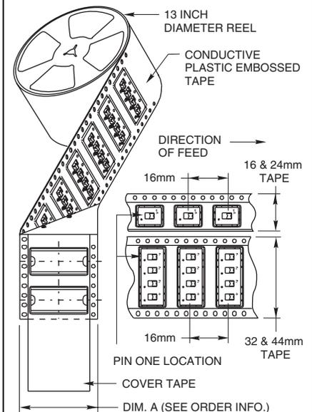
Each reel has a 15.750 inch (390 mm) minimum leader and a 6.30 inch (160 mm) minimum trailer.
