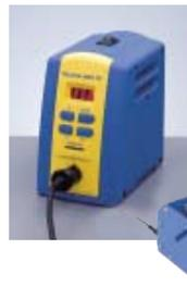
The power-save function operates while being linked to the iron holder. After the iron is inserted into the iron holder, the sleep function\*1 activates for an arbitrarily-set time (0 to 29 min.) and the tip temperature will decrease to 200°C. After 30 minutes have elapsed, the automatic power-off function\*2 activates.
