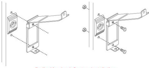
Padlocking Lock System Installation
