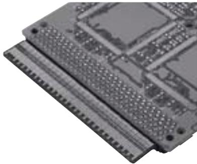
PCB through “pin-in-hole-reflow” solder technology (PIHR). It can be soldered in the same production process as the other semi finished components on the AdvancedMC™ module. Optionally, the Plug Connector
