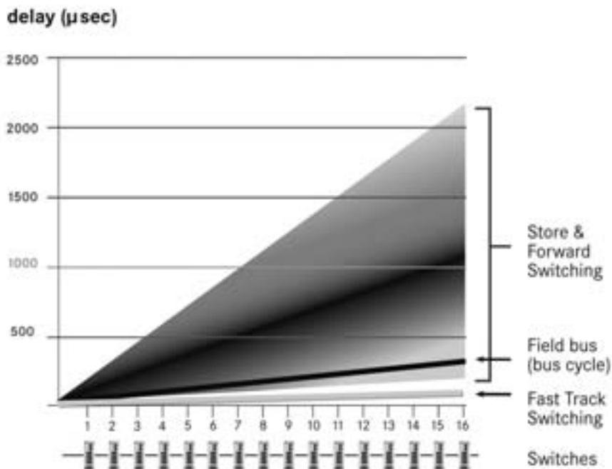
An automation frame must travel on a path through 16 switches. The transmission time for the Ethernet frames under standard switching rules is tightly dependent on the network load. Thus the transmission time for the frames can vary widely according to the network load: a few arrive quite quickly, the majority have an average time, and a few frames travel quite slowly.
