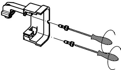
1. Pre-assemble fixing screws in the lower part
