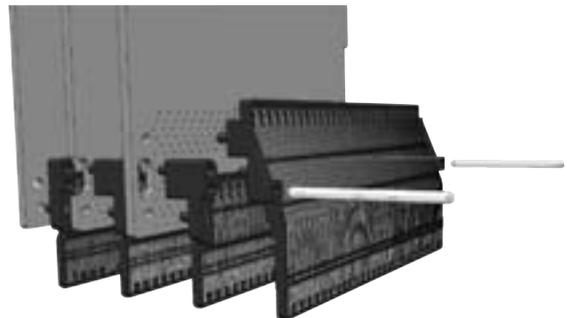
Exploded view of an MCH stack with four tongues including Piggyback Plug
