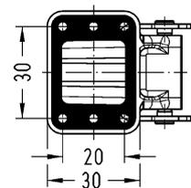
Angled bulkhead mounted housing for higher EMC requirements
