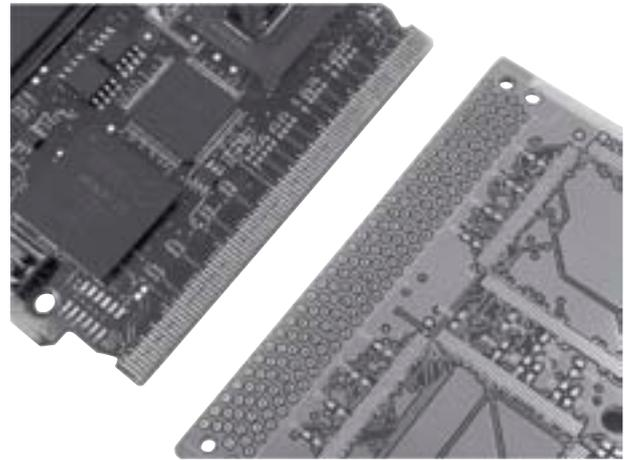
A simple board layout with through-holes is sufficient for the HARTING Plug, and these boards can be produced inexpensively and with excellent quality control, thus reducing the number of rejects. Furthermore the cost of a reject can be high if a defective PCB edge is not detected until the board is populated with expensive components. A HARTING Plug on a module can be replaced easily, reducing scrapping costs.
