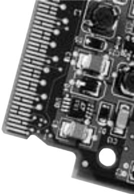
Replacing the PCB gold pads with a connector eliminates certain drawbacks of the card edge connection. The HARTING Plug Connector offers the following advantages:
