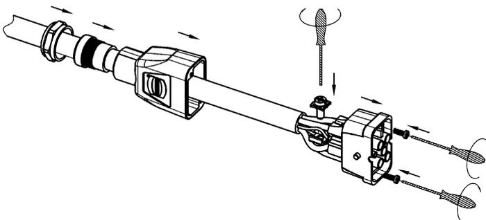
3. Connect PE conductor to the separate PE contact
