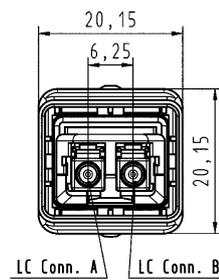
Fibre optic cable, double ended, multi mode, metal, 50 µm
