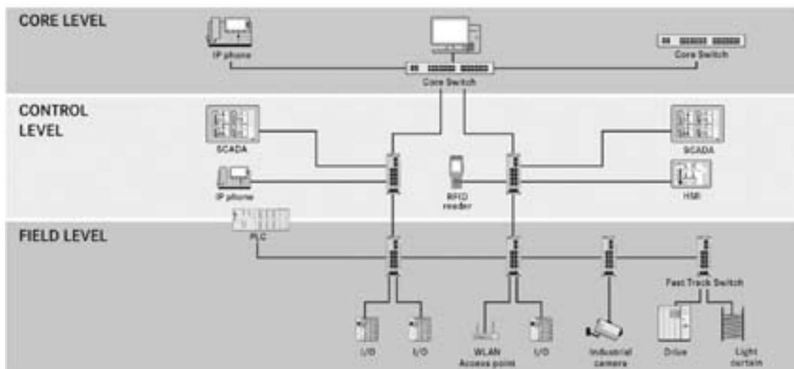
The currently available switching technology used in IEEE 802.3 Ethernet, however, does not offer the level of determinism required for automation applications. That is why automation solutions that only implement standard (unchanged) Ethernet require a restricted network design in order to match automation performance levels. Thus there are limited options for the network topology or segmentation – to the extent that IT communications are not allowed within the automation environment.
