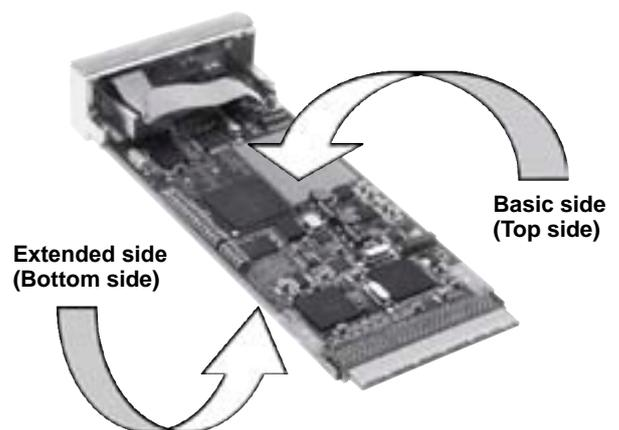
This picture shows an AdvancedMC™ module with a Plug Connector mounted on the extended side.
