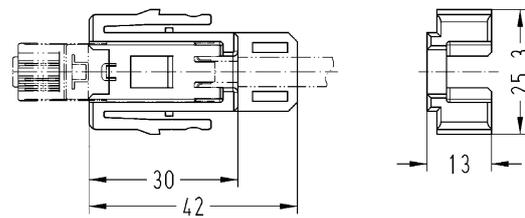
Set consists of the relevant RJ45 insert and the suitable adapter for Han® RJ45 male module 09 14 001 4623
