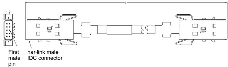
**Cable assembly har-mik® pin and socket, 68 pole**
