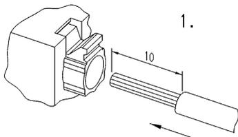
Push fine stranded wires into the Han-Quick Lock® contact and push the slide with a screw driver<sup>1)</sup> until it comes to a stop
