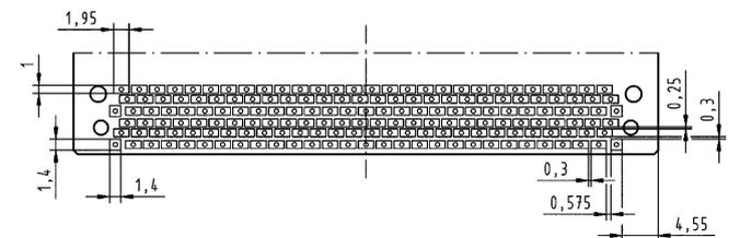
Each termination requires a solder paste volume of 0.5 mm<sup>3</sup>. Since the stencil can only provide fractions of this volume (0.29 mm<sup>3</sup> at 0.15 mm stencil thickness), the remaining solder paste must be pressed into the plated through hole. For a nominal AMC card (1.6 mm PCB thickness, 0.55 mm plated hole diameter) the paste must penetrate the hole by 0.9 mm.
