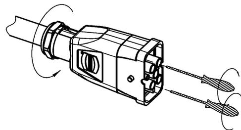
4. Fix the two parts of the hood with the pre-assembled screws and screw the cable gland
