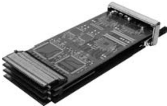
The MTCA.0 specification recommends the use of a special Plug Connector to reduce the insertion force of the module and to solve the tolerance stack-up problem between the multiple tongues and the backplane connectors.
