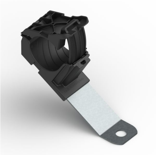
Ratchet P-Clamp, 0.76" - 1.42" Bundle Dia, 30° Long, .51" Hole Dia, PA66HIRHSUV/ST/ZN, Black, 140/ctn
