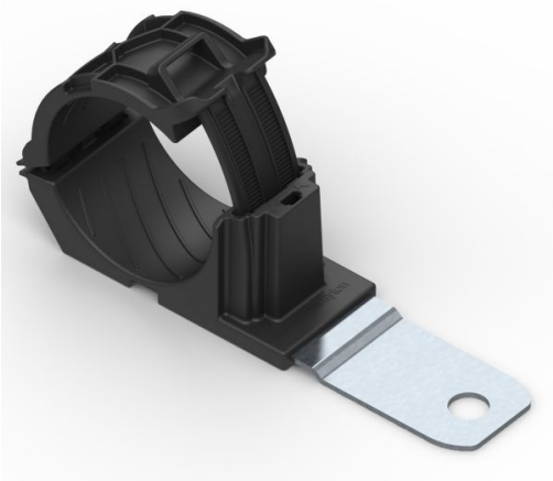
Ratchet P-Clamp, 1.38" - 2.01" Bundle Dia, 180° Med, .51" Hole Dia, PA66HIRHSUV/ST/ZN, Black, 140/ctn
