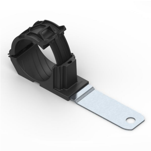
Ratchet P-Clamp, 1.38" - 2.01" Bundle Dia, 180° Long, .41" Hole Dia, PA66HIRHSUV/ST/ZN, Black, 140/ctn
