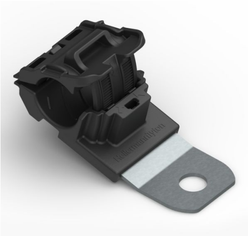
Ratchet P-Clamp, 0.52" - 0.77" Bundle Dia, 15° Short, .26" Hole Dia, PA66HIRHSUV/SS304, Black, 280/ctn
