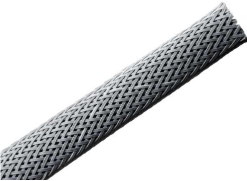
Braided Sleeving, Expandable, Flame Retardant, 0.25" Dia, PET, Gray, 200 ft/reel
