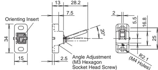
The orientation of actuator adjustment (horizontal/vertical) can be changed using the orienting insert (white plastic) installed on the back of the actuator.
