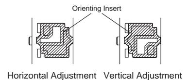
Note: The base is made of glass-reinforced PA66 (66 nylon). Angle adjustment screws are stainless steel. When using adhesive on screws, take material compatibility into consideration.
