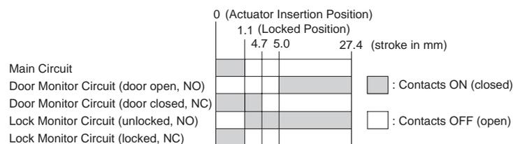
• The characteristics shown in the chart above are of the HS9Z-A61, -A62, -A65, and -A66 actuators. For HS9Z-A62S actuator, subtract 0.6 mm.
