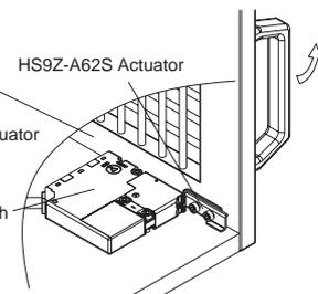
Note: When mounting an actuator, make sure that the actuator enters the slot in the correct direction, as shown on the right.
