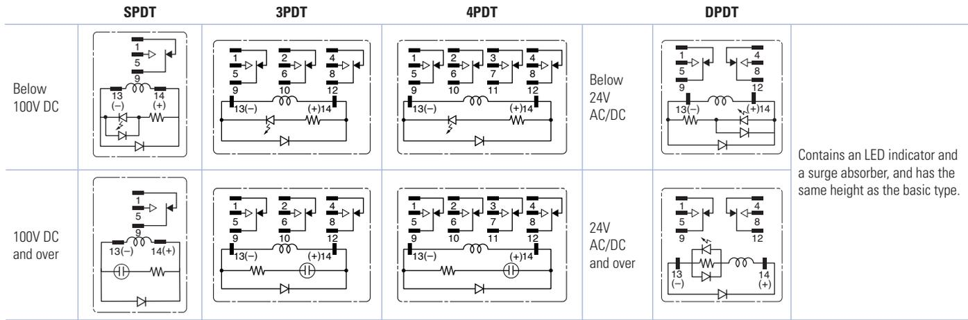
Contains an LED indicator and a surge absorber, and has the same height as the basic type.
