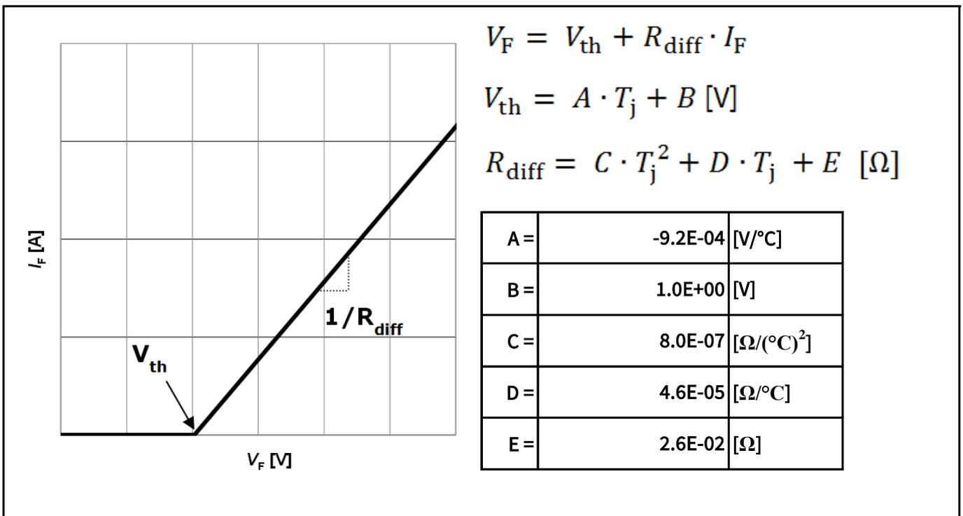
Figure 6 Simplified forward characteristics model  $V_F = f(I_F)$ ;
