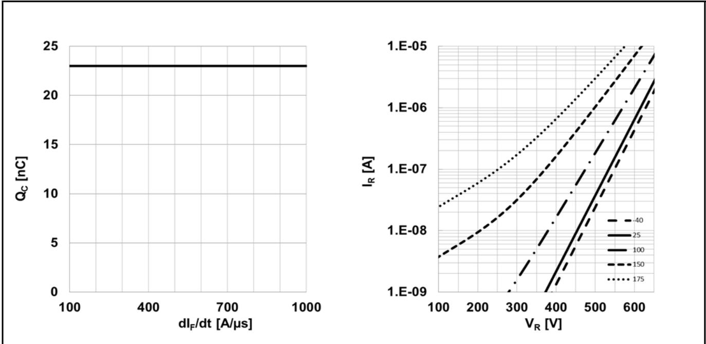
Figure 3 (LEFT) Typical capacitive charge versus current slope (only capacitive charge, guaranteed by design);  $Q_c = f(di_F/dt)$ ;  $T_j = 150^\circ\text{C}$ ;  $V_R = 400\text{V}$ ;  $I_F \leq I_{F,max}$
