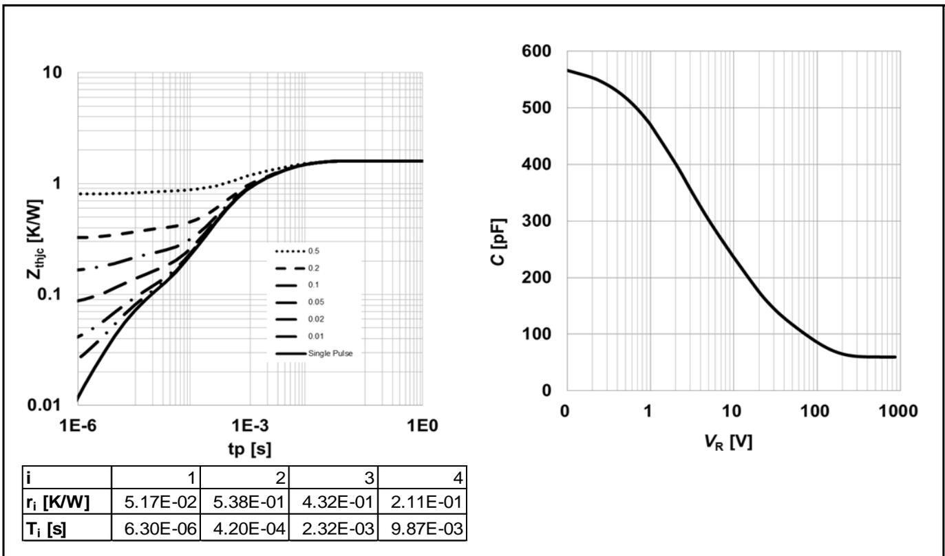
Figure 4 (LEFT) Max. Transient thermal impedance;  $Z_{thjc} = f(t_p)$ ; parameter:  $D = t_p/T$
