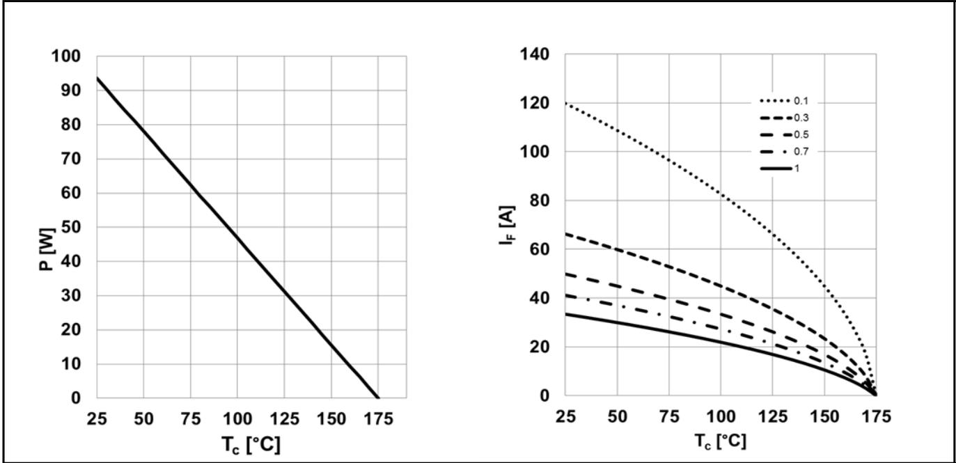
Figure 1 (LEFT) Power dissipation;  $P_{tot} = f(T_C)$ ;  $R_{thJC,max}$
