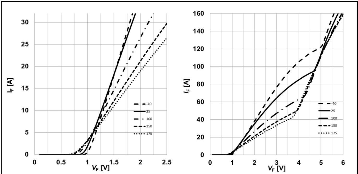
Figure 2 (LEFT) Typical forward characteristic;  $I_F = f(V_F)$ ;  $t_p = 200\text{ }\mu\text{s}$ ; parameter:  $T_j$
