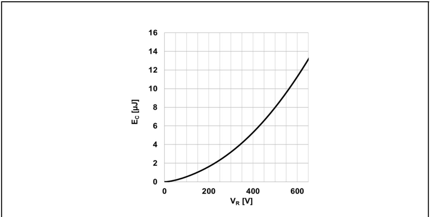
Figure 5 Typical capacitance stored energy;  $E_c = f(V_R)$
