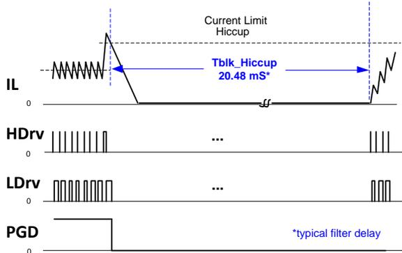
Figure 9: Timing Diagram for Current Limit Hiccup
