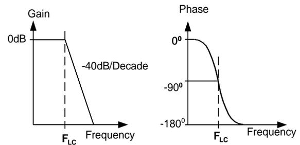
Figure 25: Gain and Phase of LC filter
