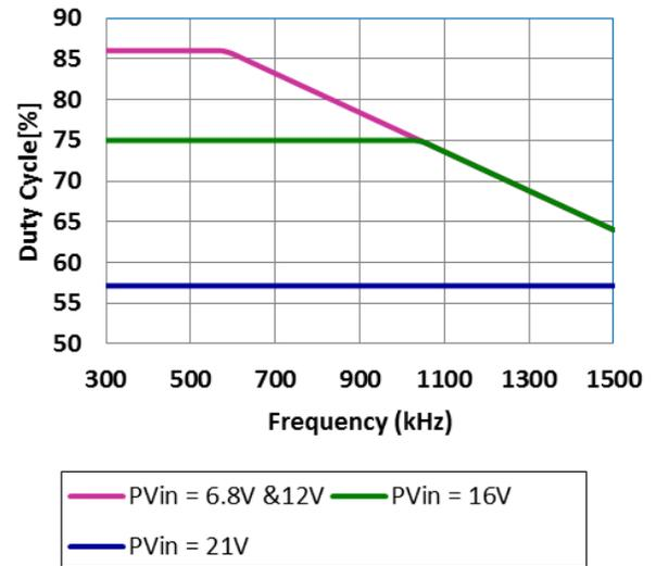
Figure 21: Maximum duty cycle vs. switching frequency
