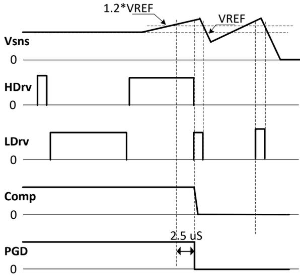
Figure 20: Timing Diagram for OVP in non-tracking mode
