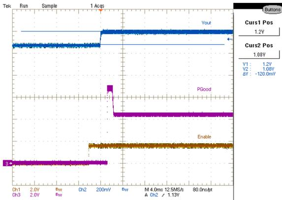
Figure 33: Vout Startup with Pre-Bias, 1.08V
