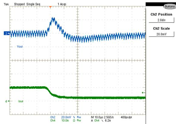
Figure 37:  $V_{out}$  Transient Response, 2.5A to 10.0A step at 2.5A/uSec
