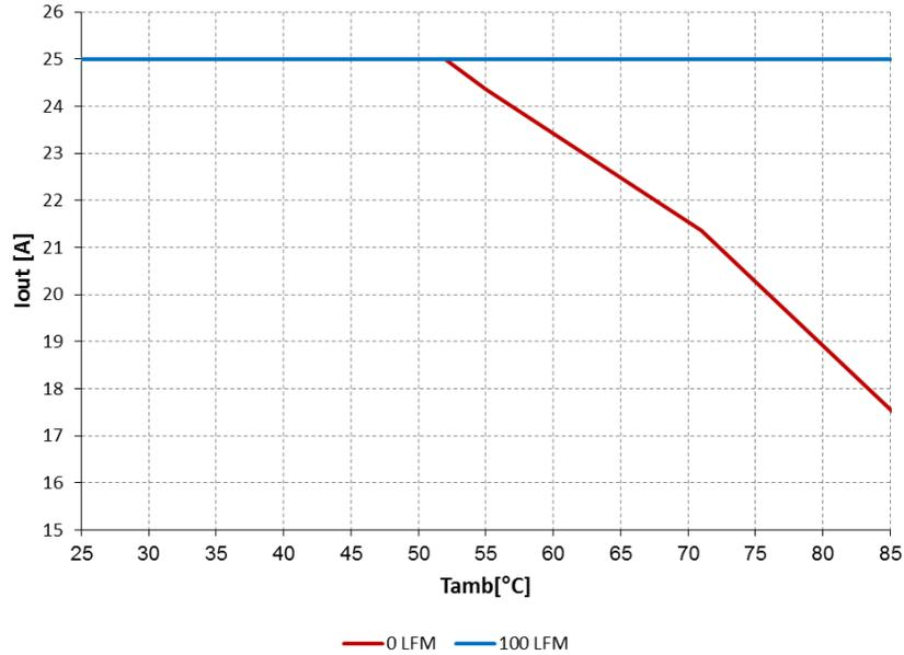
$V_{in}=P_{Vin}=12V$ ,  $V_{out}=5.0V$ ,  $V_{CC}=\text{internal LDO (6.8V)}$ ,  $F_s = 600kHz$
