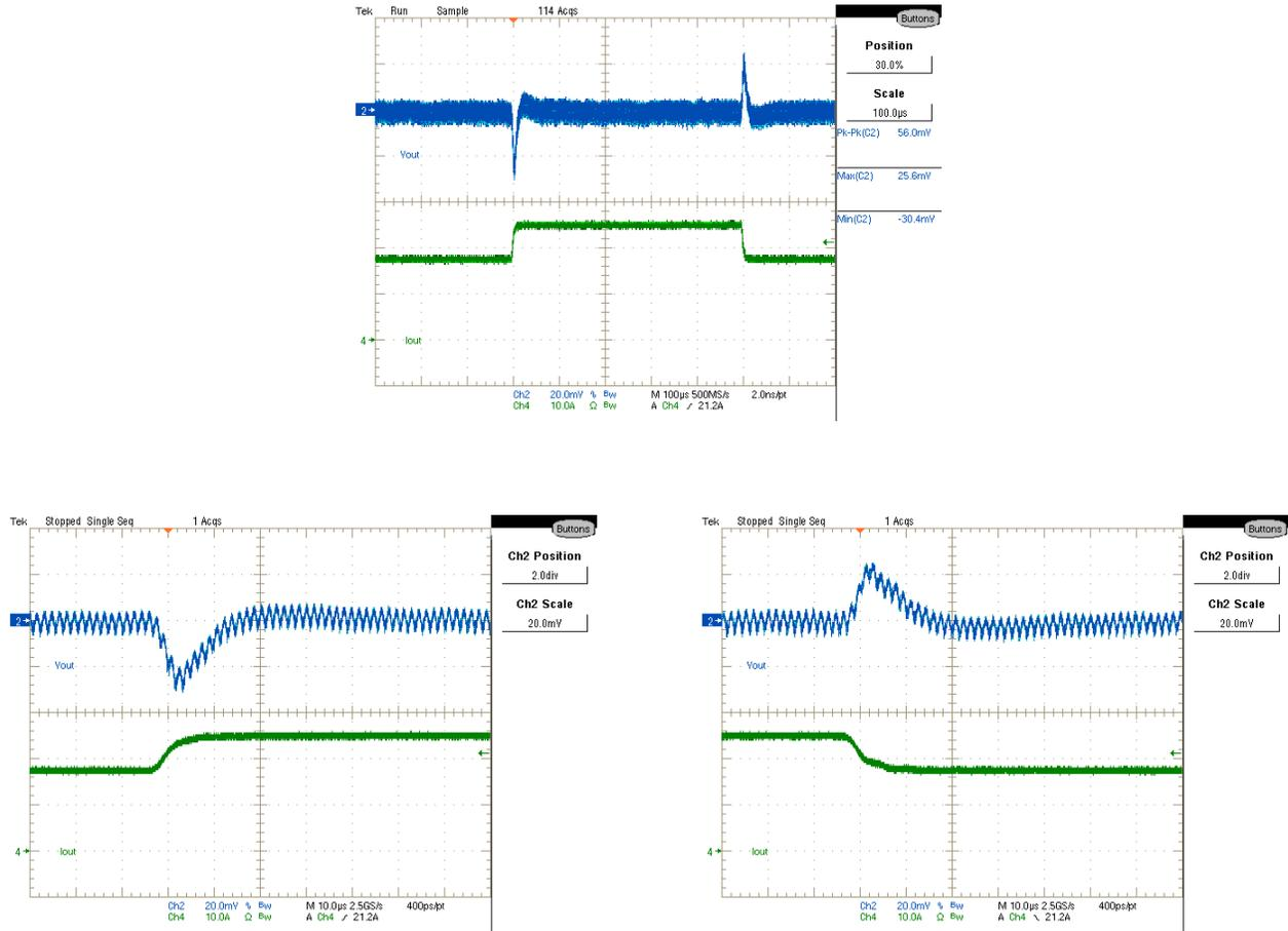
Figure 38:  $V_{out}$  Transient Response, 17.5A to 25A step at 2.5A/µSec
