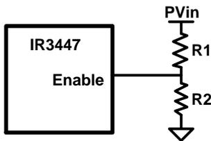
Figure 22: Using Enable pin for UVLO implementation
