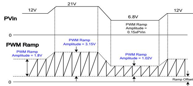
Figure 13: Timing Diagram for Feed-Forward (F.F.) Function
