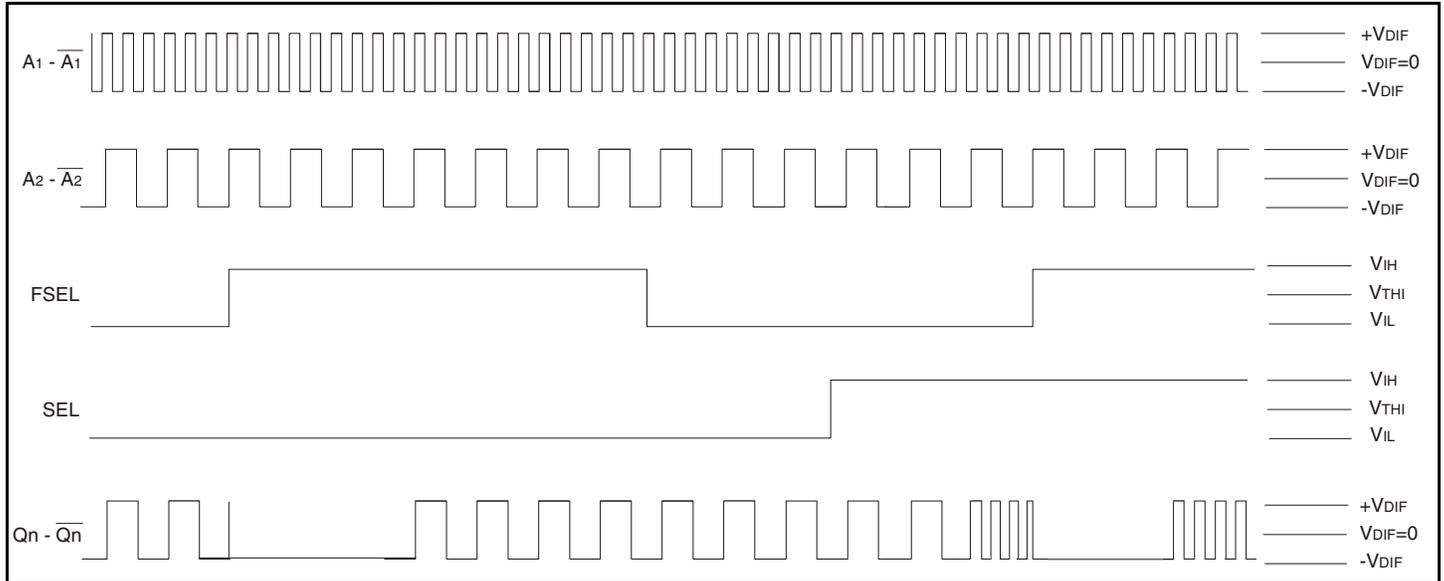
1. If the user holds FSEL HIGH, the output will not be affected by the deselected input clock.
