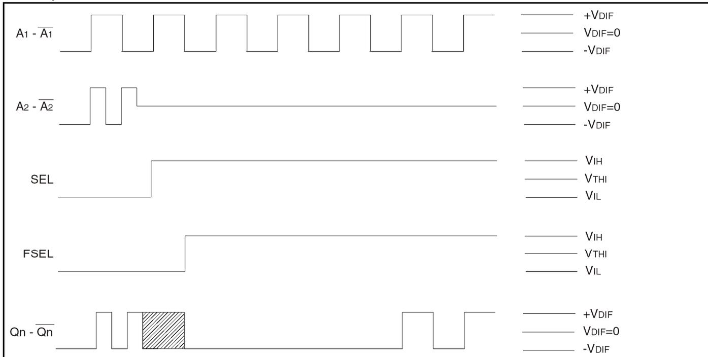
1. When the differential on the selected clock goes below the minimum DC differential, the outputs clock goes to an unknown state. When this happens, the SEL pin should be toggled and FSEL asserted in order to force selection of the new input clock. The output clock will start up after a number of cycles of the newly-selected input clock.
