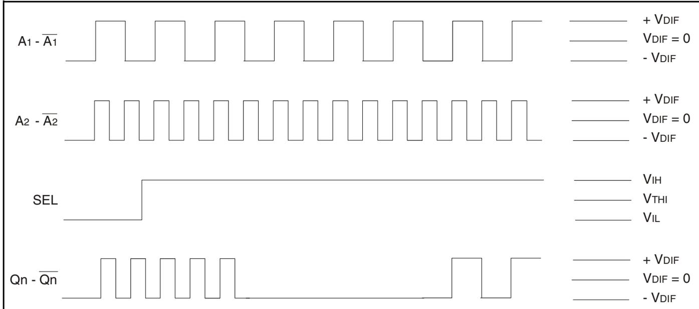
1. When SEL changes, the output clock goes LOW on the falling edge of the output clock up to three cycles later. The output then stays LOW for up to three clock cycles of the new input clock. After this, the output starts with the rising edge of the new input clock.
