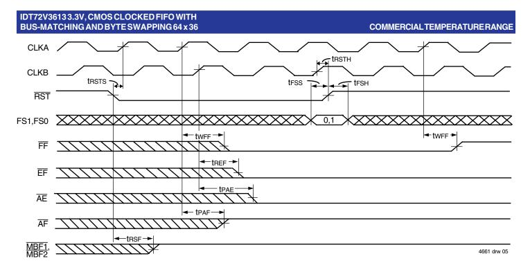
Figure 5. FIFO Reset and Loading the X Register with the Value of Eight
