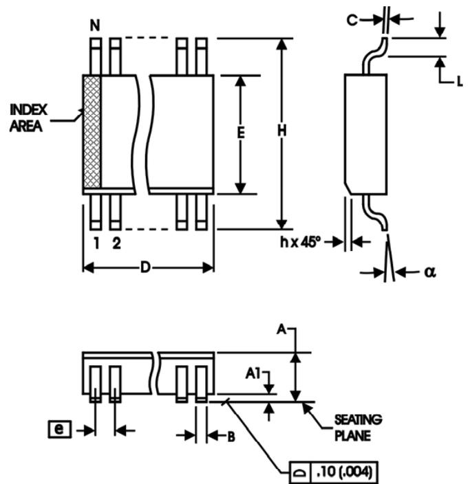
Table 9B. Package Dimensions for 16 Lead SOIC
