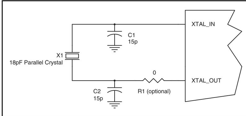
Figure 2. Crystal Input Interface
