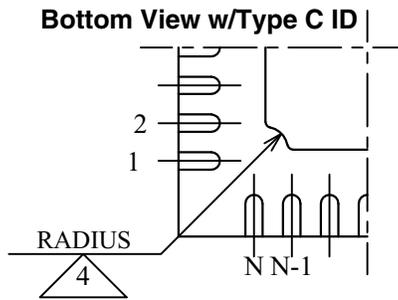
There are 2 methods of indicating pin 1 corner at the back of the VFQFN package:
