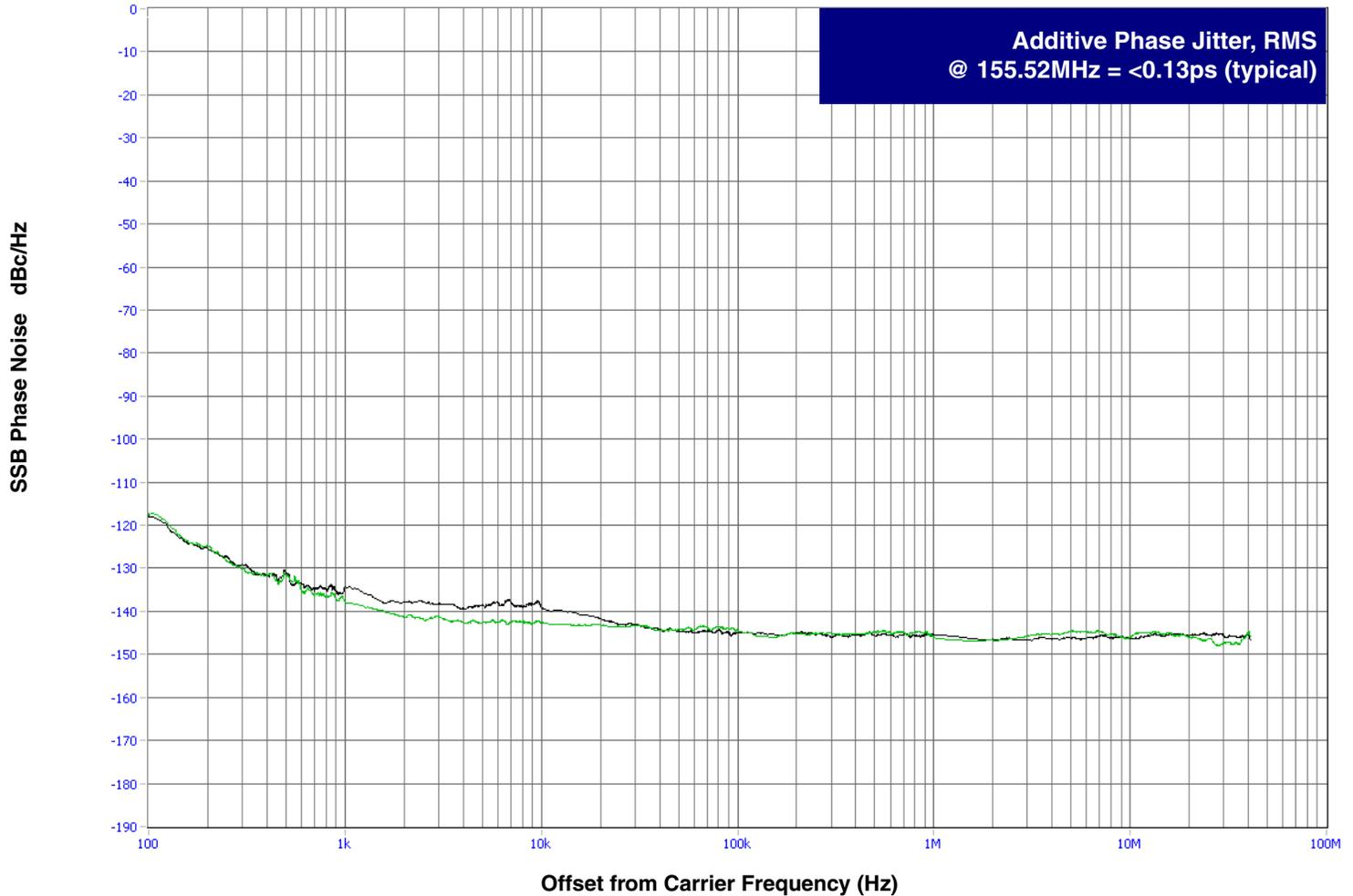
As with most timing specifications, phase noise measurements has issues relating to the limitations of the equipment. Often the noise floor of the equipment is higher than the noise floor of the device. This
