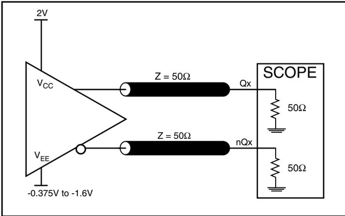
Output Load Test Circuit
