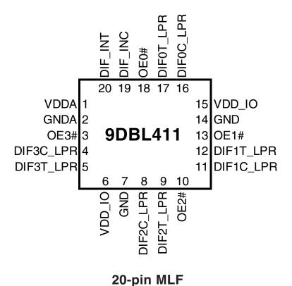
IDT® Four Output Differential Buffer for PCI Express
