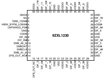
Note: Pins with ^ prefix have internal 120K pullup Pins with v prefix have internal 120K pulldowm
