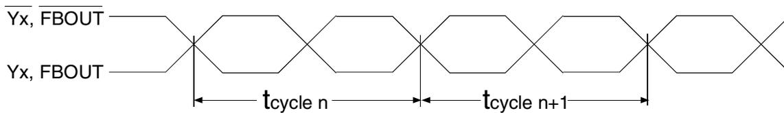
$$t_{jit(cc)} = t_{cycle\ n} - t_{cycle\ n+1}$$
