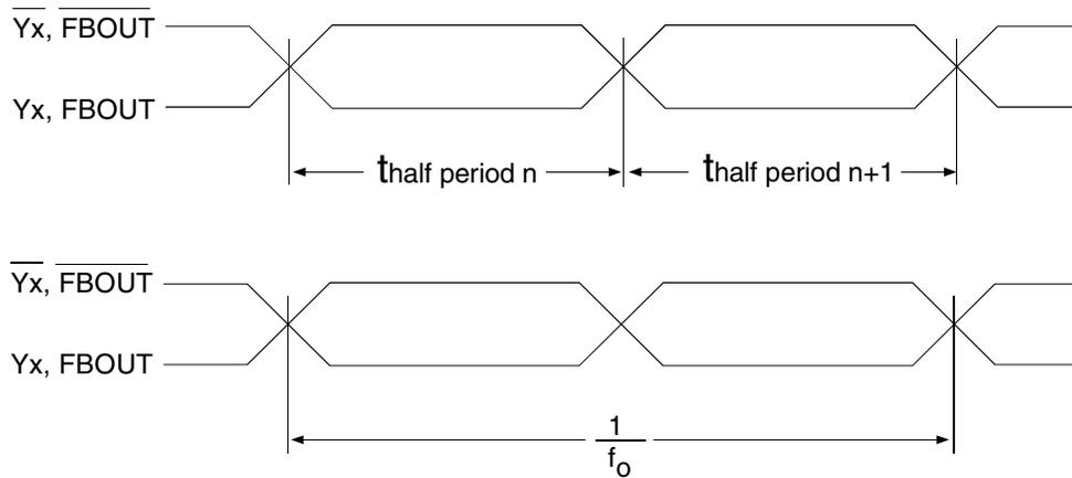
$$t_{\text{jit(hper)}} = t_{\text{half period } n} - \frac{1}{2 \cdot f_0}$$
