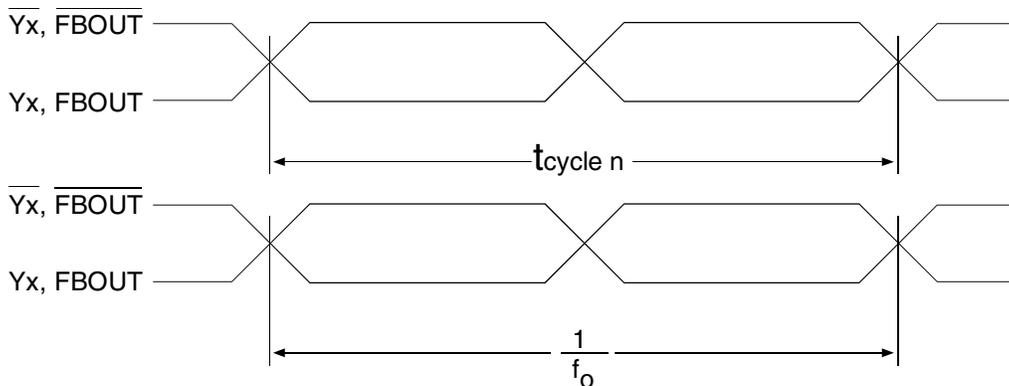
$$t_{\text{jit(per)}} = t_{\text{cycle } n} - \frac{1}{f_0}$$
