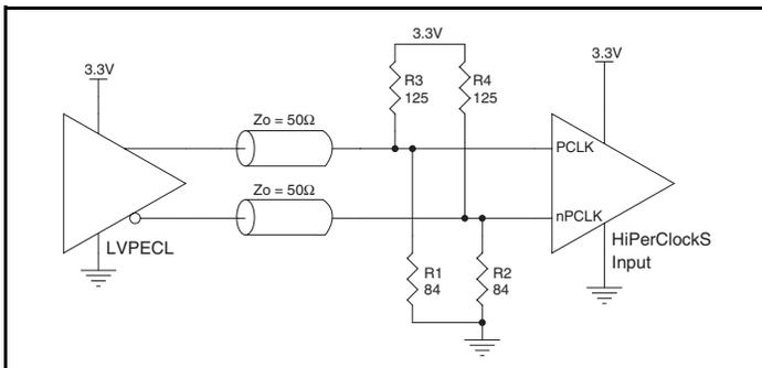
**Figure 2C. HiPerClockS PCLK/nPCLK Input Driven by a 3.3V LVPECL Driver**
