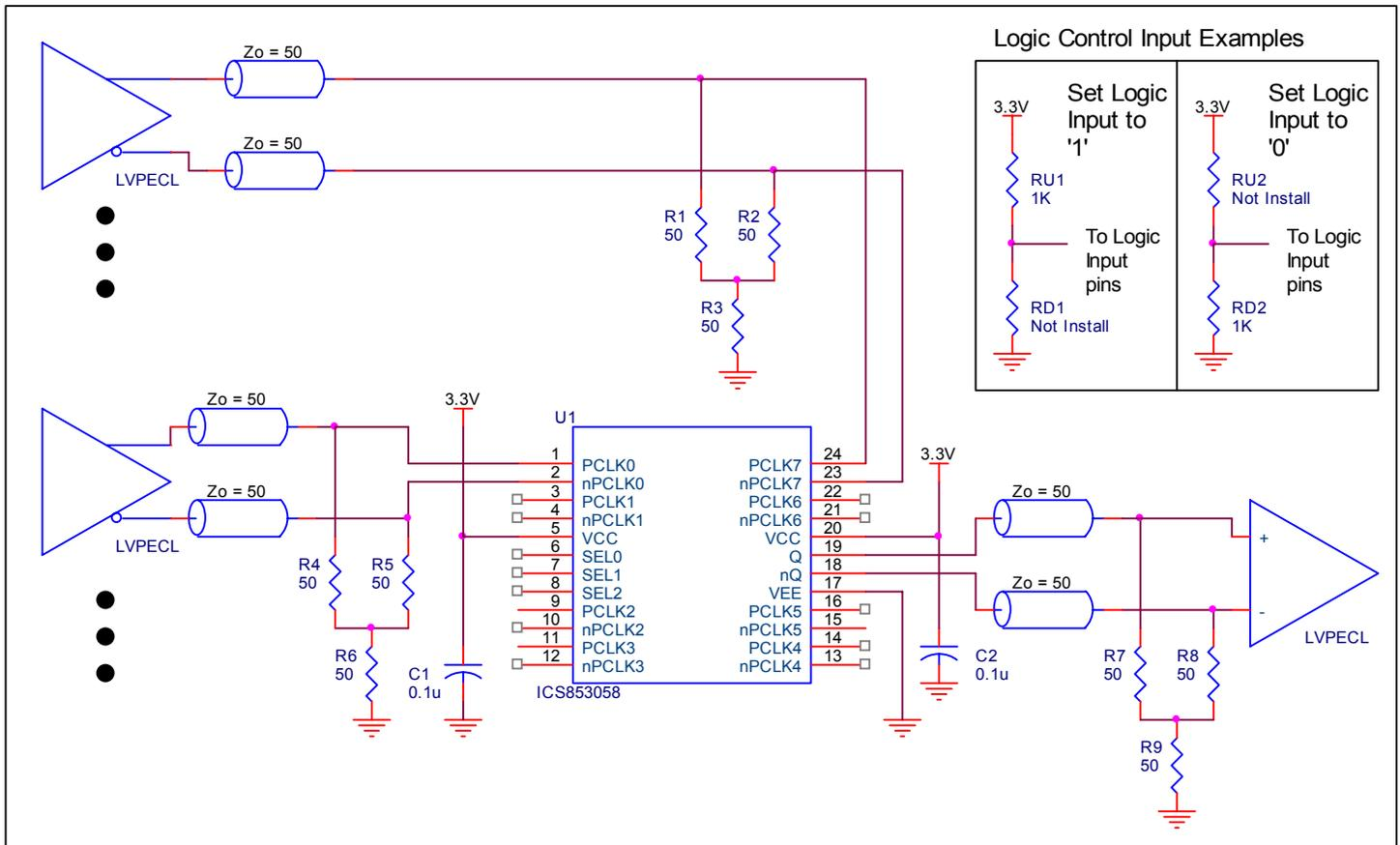
Figure 5. ICS853058 Schematic Example
