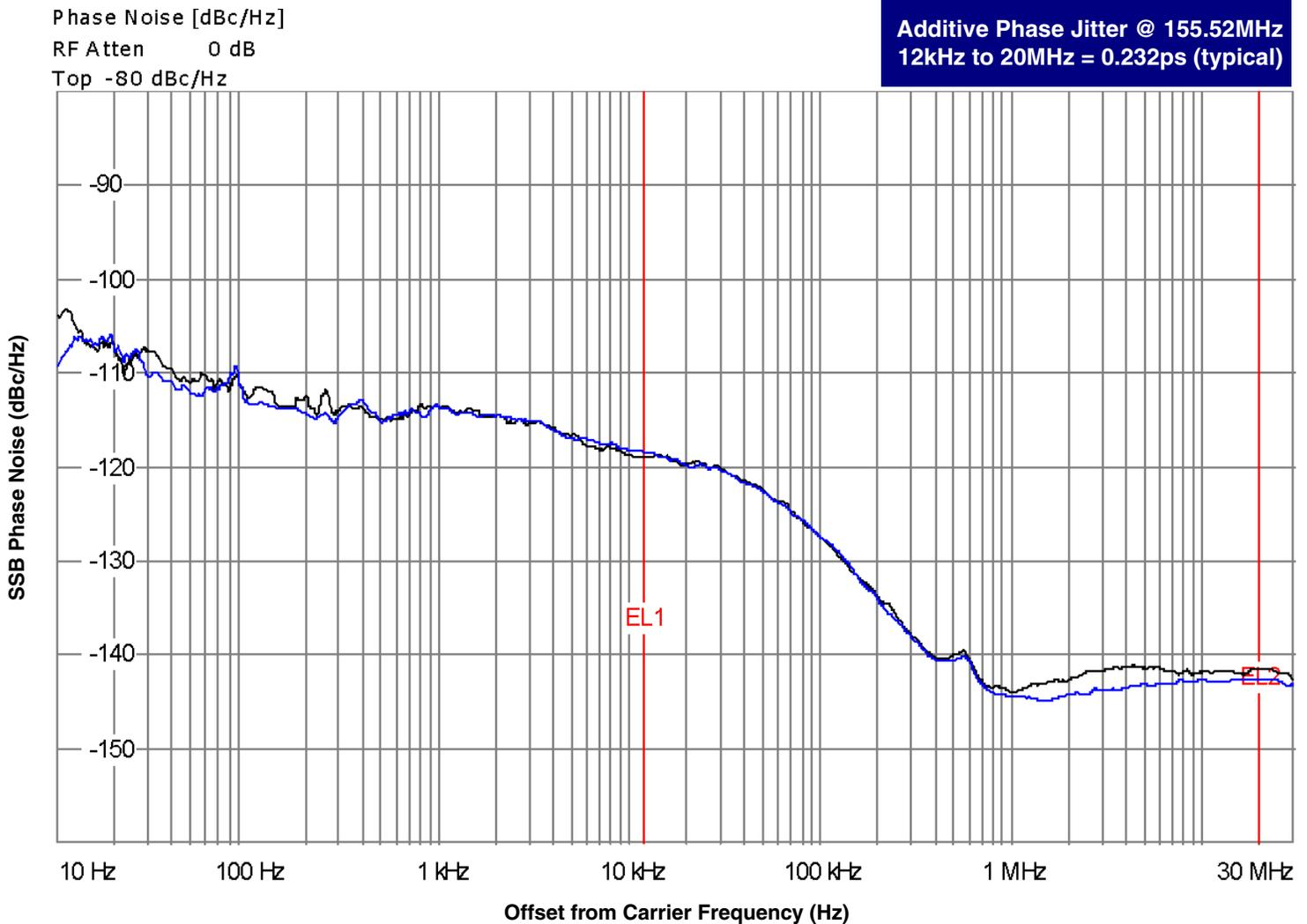
As with most timing specifications, phase noise measurements has issues relating to the limitations of the equipment. Often the noise floor of the equipment is higher than the noise floor of the device. This
