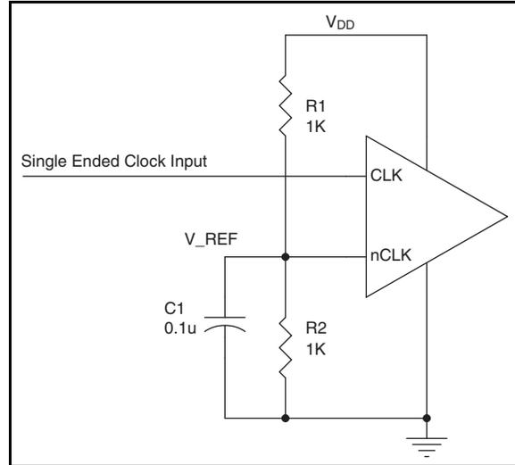
Figure 1. Single-Ended Signal Driving Differential Input
