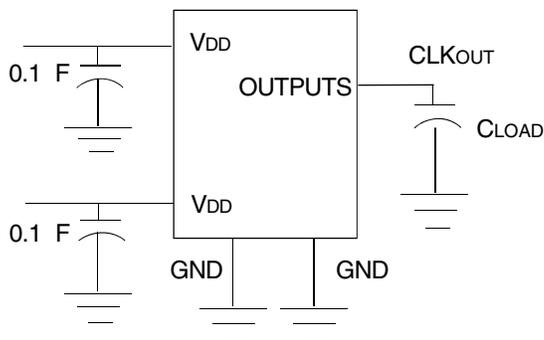
Test Circuit 1 (all Parameters Except  $t_8$ )
