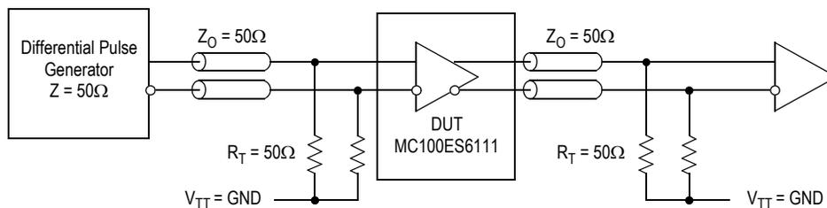
**Figure 3. MC100ES6111 AC Test Reference**
