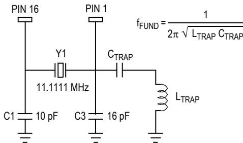
**Figure 4. Crystal Oscillator Interface
