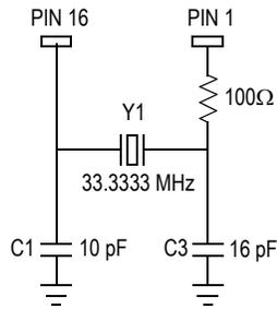
**Figure 3. Crystal Oscillator Interface
