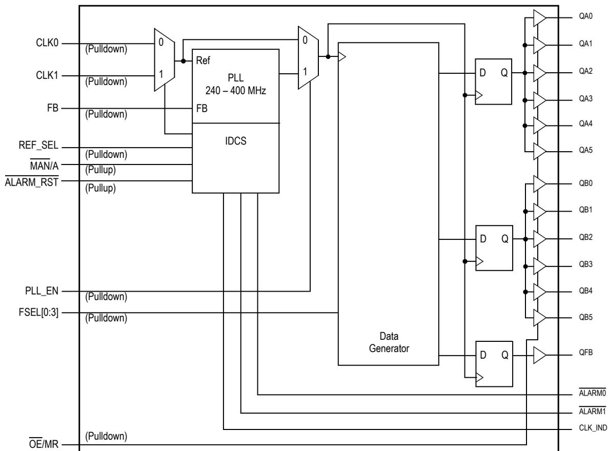
Figure 1. MPC9893 Logic Diagram
