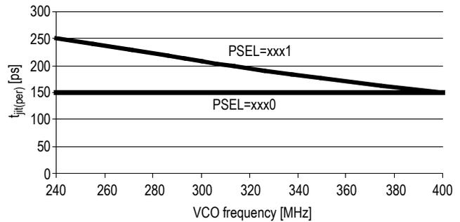
Figure 7. Max. Period Jitter versus VCO Frequency
