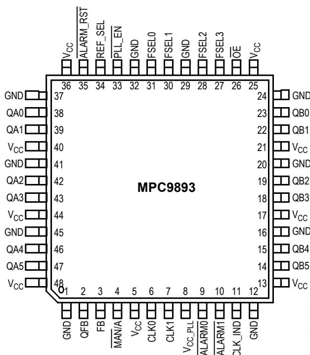
It is recommended to use an external RC filter for the analog power supply pin V<sub>CC\_PLL</sub>. Please see application section for details.
