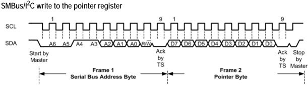
SMBus/I<sup>2</sup>C write to the pointer register followed by a write data word
