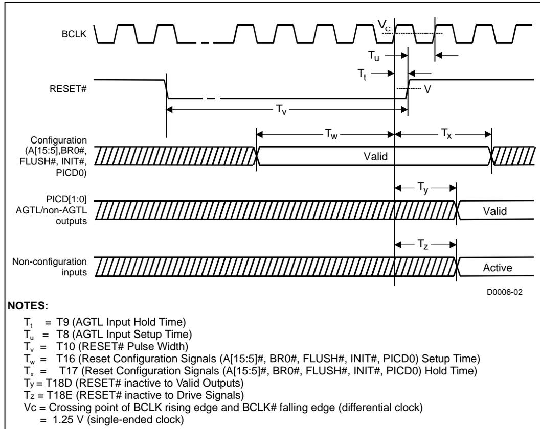
Figure 16. Power-On Sequence and Reset Timings
