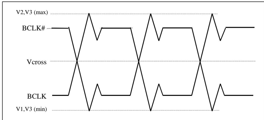
Figure 12. BCLK/BCLK# Waveform (Differential Mode)
