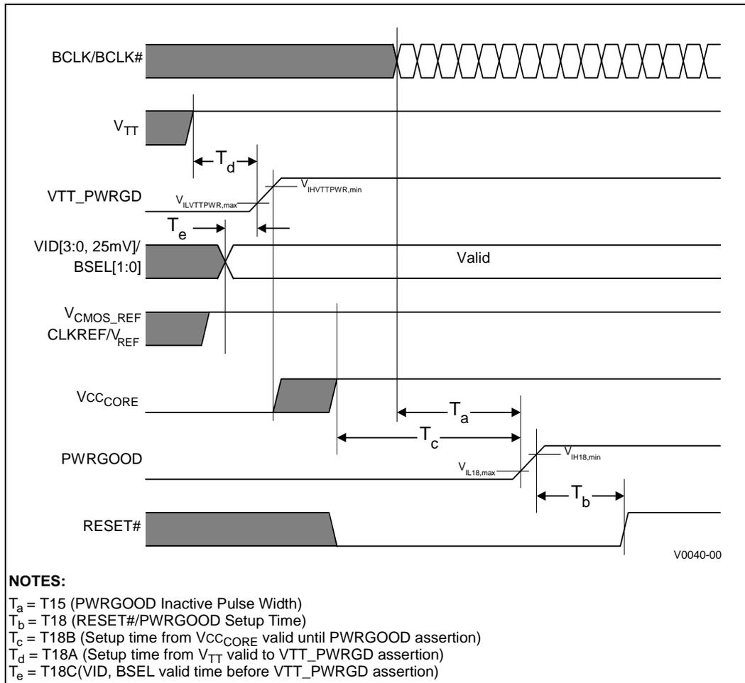
Figure 17. Test Timings (Boundary Scan)
