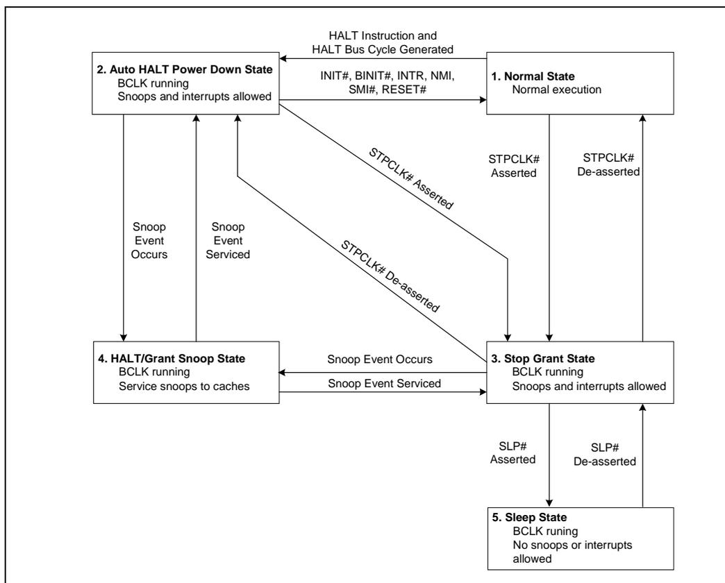
For the processor to fully realize the low current consumption of the Stop-Grant and Sleep states, a Model Specific Register (MSR) bit must be set. For the MSR at 02AH (Hex), bit 26 must be set to a '1' (this is the power on default setting) for the processor to stop all internal clocks during these modes. For more information, see the *Intel Architecture Software Developer's Manual, Volume 3: System Programming Guide*.
