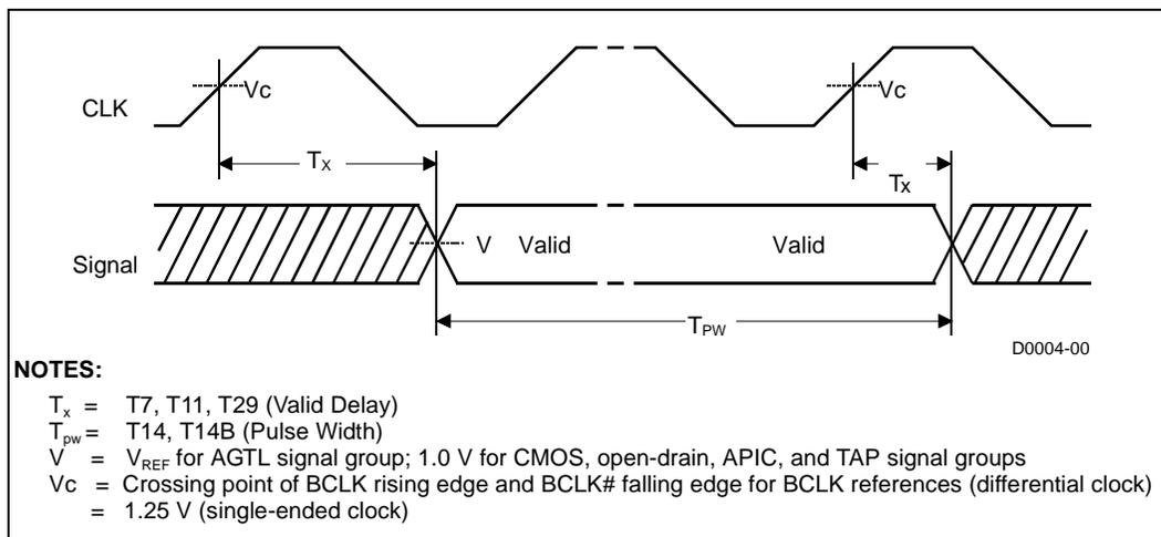
Figure 14. Setup and Hold Timings
