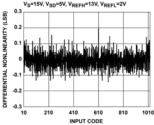
FIGURE 1. DIFFERENTIAL NONLINEARITY vs CODE
