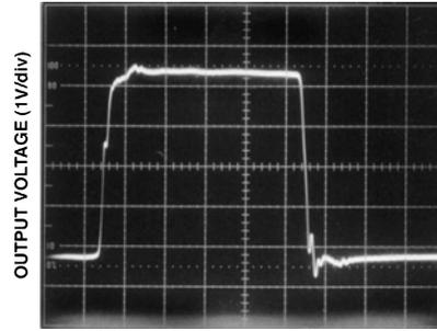
$V_S = \pm 5V$   $R_F = R_G = 750\Omega$   $R_L = 150\Omega$   $A_V = +2$
