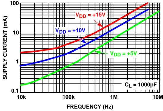
FIGURE 7. AVERAGE SUPPLY CURRENT vs VOLTAGE AND FREQUENCY
