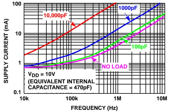
FIGURE 8. AVERAGE SUPPLY CURRENT vs CAPACITIVE LOAD
