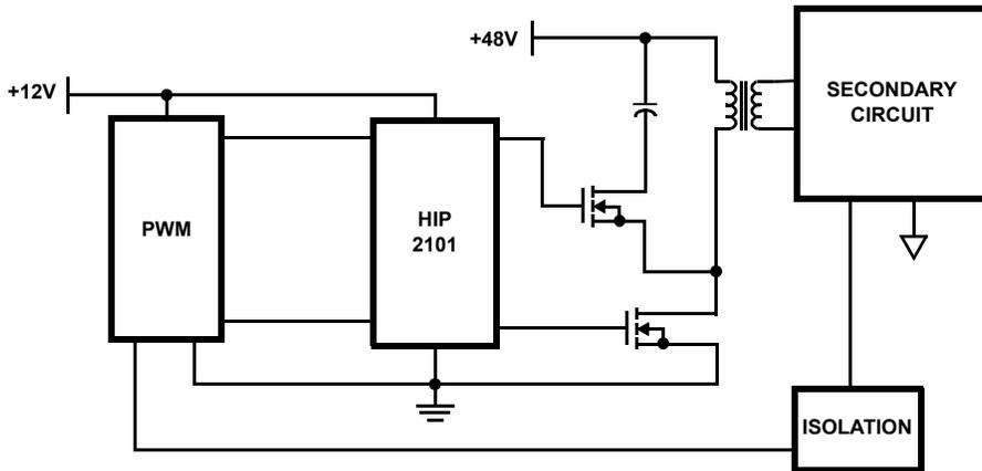
FIGURE 2. FORWARD CONVERTER WITH AN ACTIVE CLAMP
