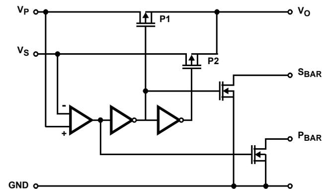
$V_P > V_S$ , P1 SWITCH ON AND P<sub>BAR</sub> SWITCH ON
