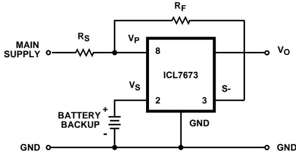
FIGURE 12. LOW CURRENT BATTERY BACKUP SYSTEM WITH HYSTERESIS
