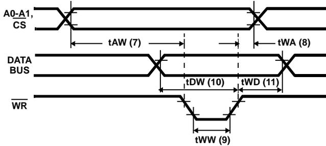
FIGURE 30. WRITE TIMING
