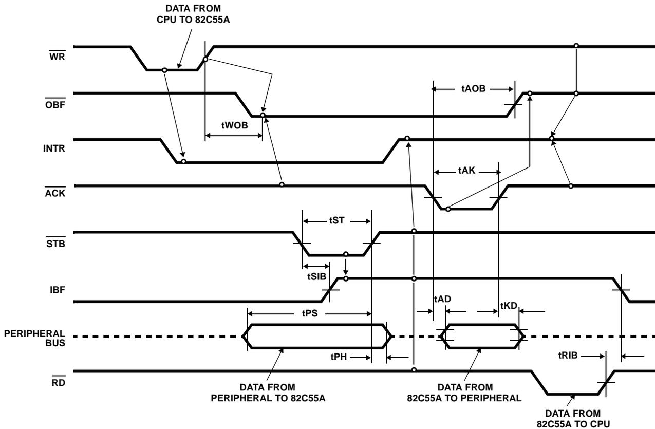
NOTE: Any sequence where  $\overline{WR}$  occurs before  $\overline{ACK}$  and  $\overline{STB}$  occurs before  $\overline{RD}$  is permissible. ( $INTR = IBF \cdot MASK \cdot \overline{STB} \cdot \overline{RD} + \overline{OBF} \cdot MASK \cdot \overline{ACK} \cdot \overline{WR}$ )
