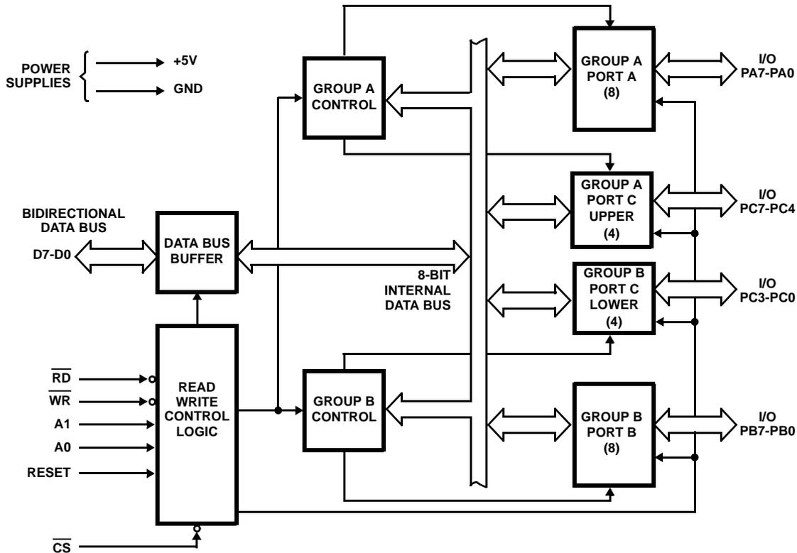
FIGURE 1. FUNCTIONAL DIAGRAM
