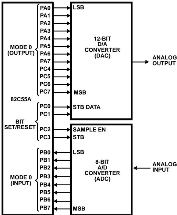
FIGURE 21. DIGITAL TO ANALOG, ANALOG TO DIGITAL
