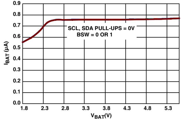
FIGURE 2.  $I_{BAT}$  vs  $V_{BAT}$ , SBIB = 1
