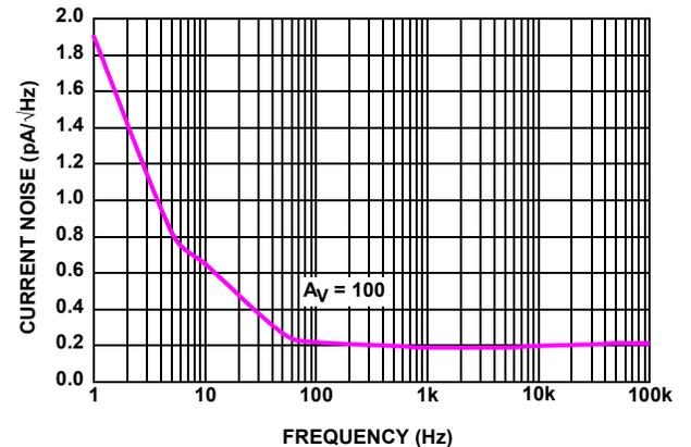
FIGURE 18. ISL28272 INPUT CURRENT NOISE SPECTRAL DENSITY
