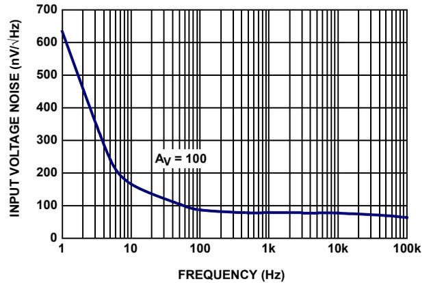
FIGURE 16. ISL28272 INPUT VOLTAGE NOISE SPECTRAL DENSITY
