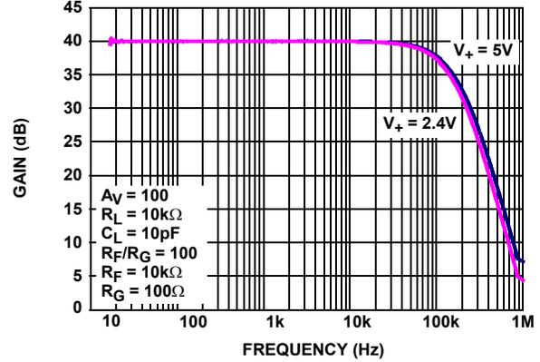
FIGURE 8. ISL28272 FREQUENCY RESPONSE vs SUPPLY VOLTAGE
