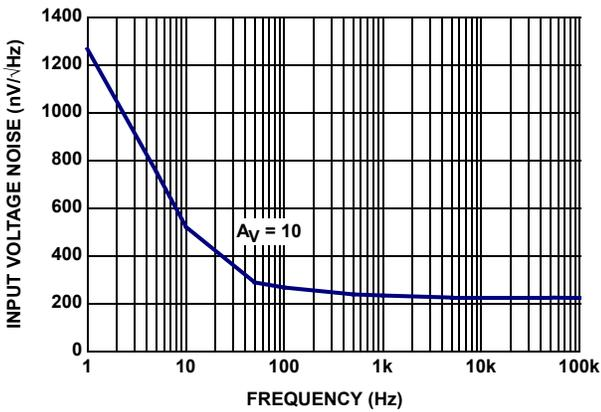
FIGURE 15. ISL28271 INPUT VOLTAGE NOISE SPECTRAL DENSITY
