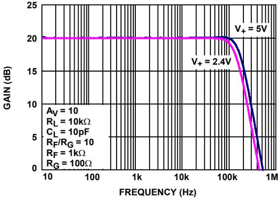
FIGURE 7. ISL28271 FREQUENCY RESPONSE vs SUPPLY VOLTAGE
