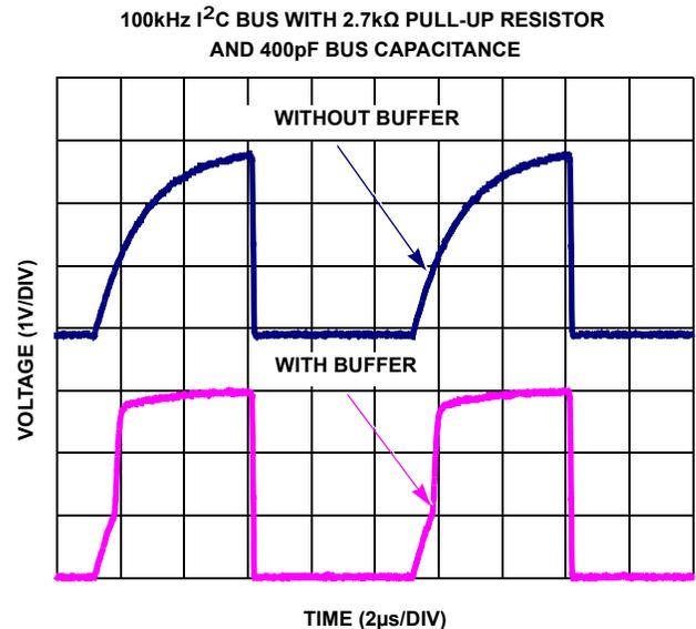
FIGURE 2. BUS ACCELERATOR PERFORMANCE
