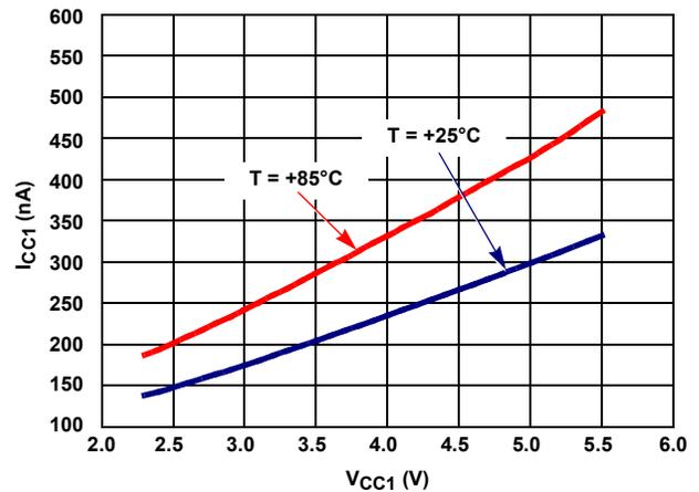
FIGURE 12.  $I_{CC1}$  DISABLED CURRENT vs  $V_{CC1}$  (ISL33001)
