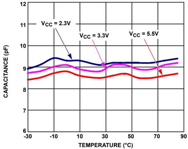
FIGURE 25. SDA/SCL PIN CAPACITANCE vs TEMPERATURE vs  $V_{CC}$
