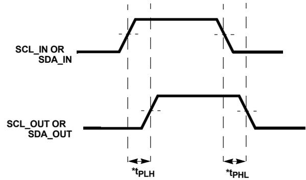
\*Propagation delay measured between 50% of  $V_{CC1}$
