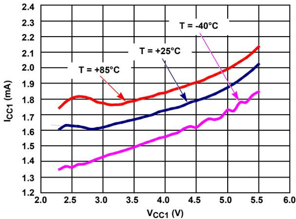
FIGURE 11.  $I_{CC1}$  ENABLED CURRENT vs  $V_{CC1}$  (ISL33001)
