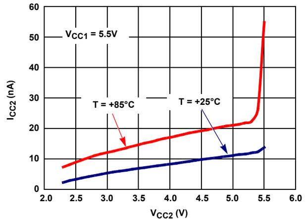
FIGURE 16.  $I_{CC2}$  DISABLED CURRENT vs  $V_{CC2}$  (ISL33003)
