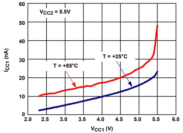
FIGURE 14.  $I_{CC1}$  DISABLED CURRENT vs  $V_{CC1}$  (ISL33003)
