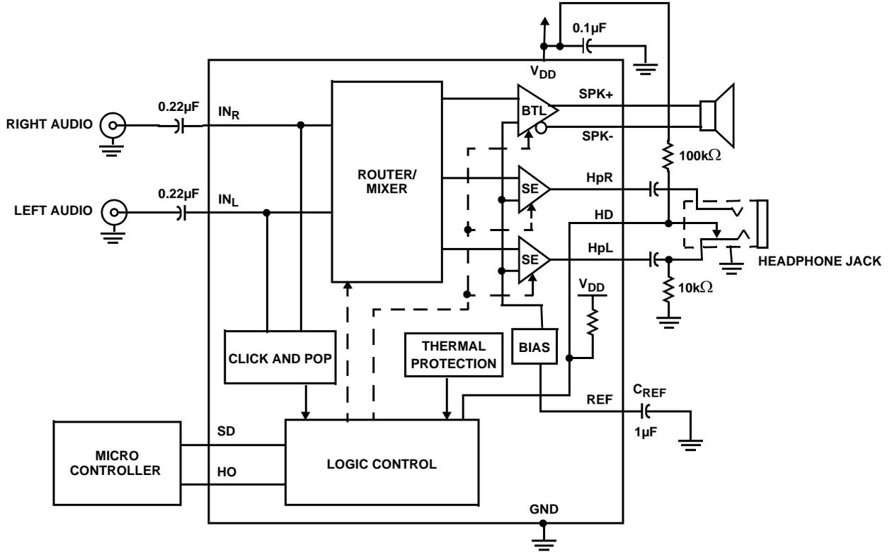
**ISL54005 Typical Application Circuit and Block Diagram**
