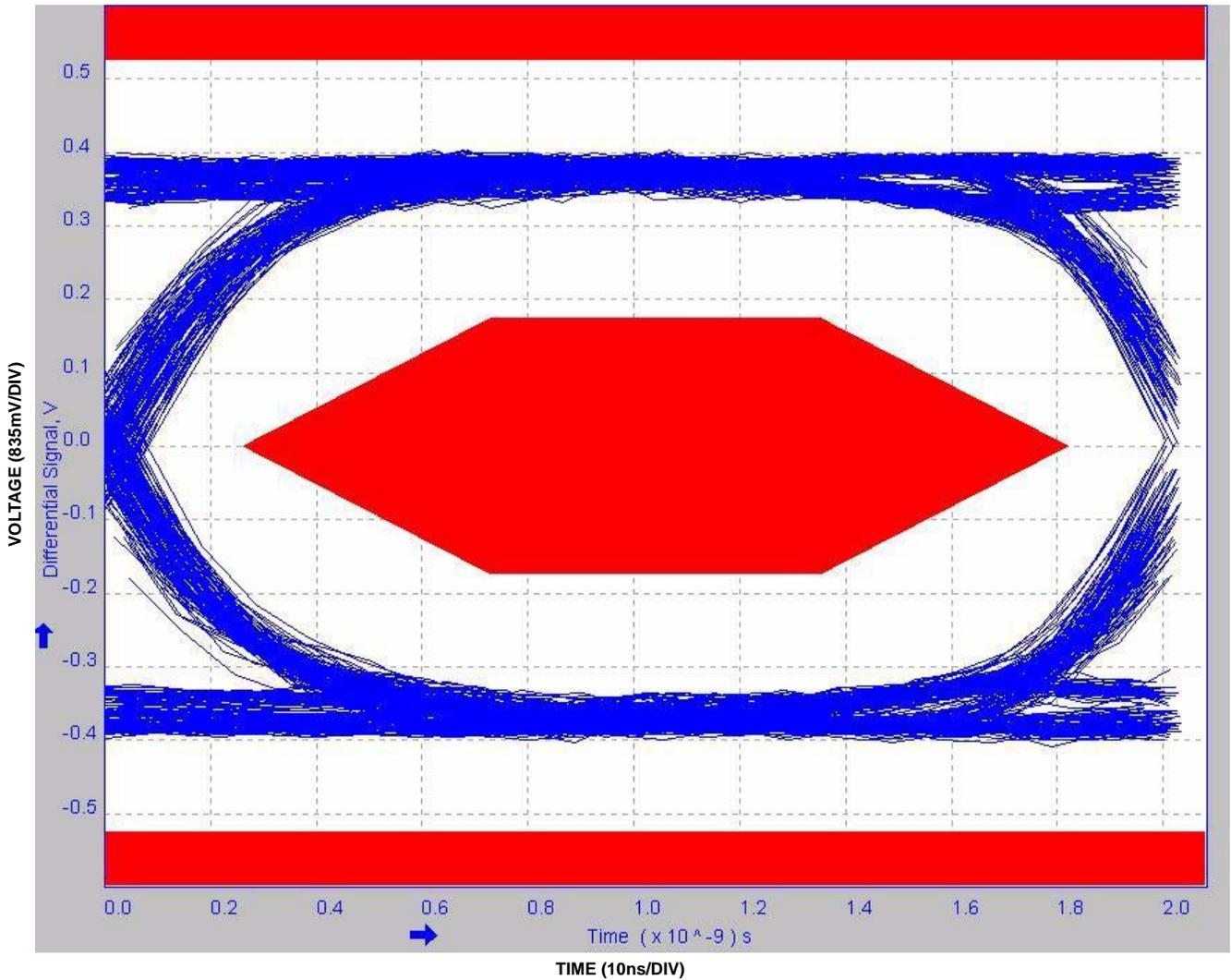
FIGURE 14. EYE PATTERN: 480Mbps WITH NO<sub>x</sub> SWITCHES IN THE SIGNAL PATH
