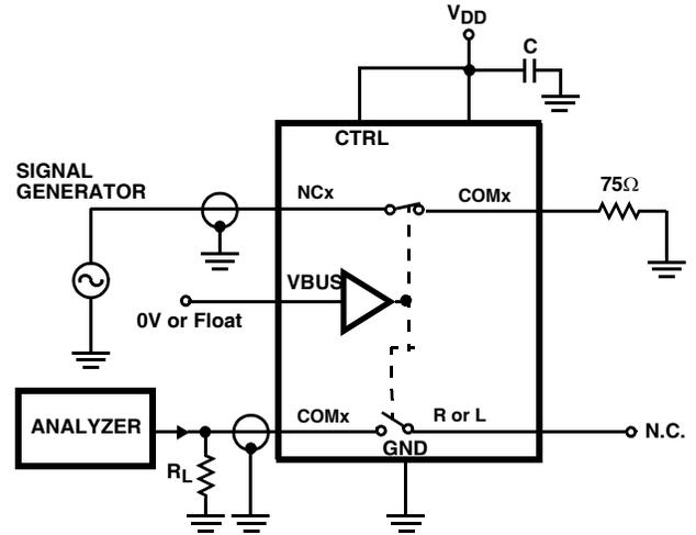
FIGURE 6. AUDIO CROSTALK TEST CIRCUIT
