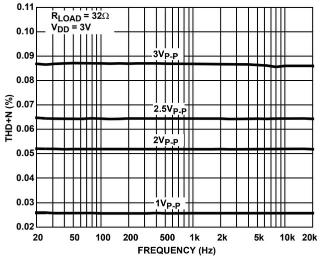
FIGURE 12. THD+N vs SIGNAL LEVELS vs FREQUENCY
