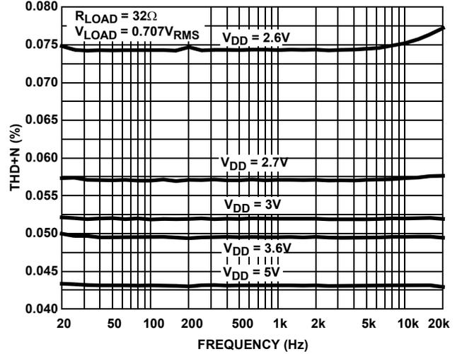
FIGURE 11. THD+N vs SUPPLY VOLTAGE vs FREQUENCY
