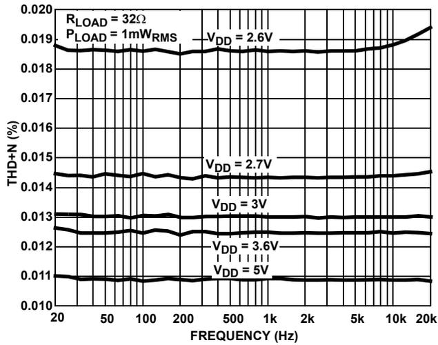
FIGURE 10. THD+N vs SUPPLY VOLTAGE vs FREQUENCY
