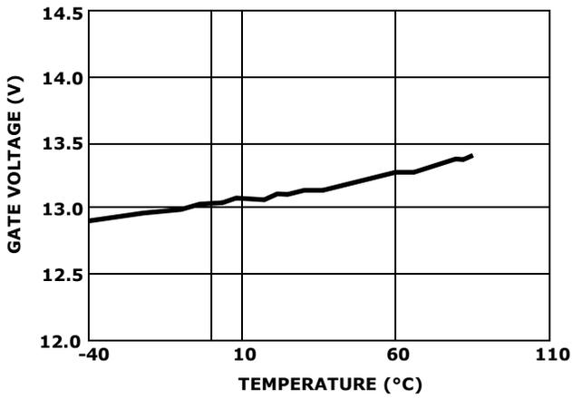
FIGURE 16. GATE VOLTAGE (AT  $V_{DD} = 17V$ )
