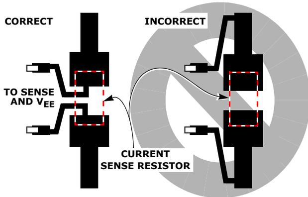
FIGURE 5. SENSE RESISTOR
