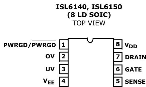
ISL6140 has active Low (L version)  $\overline{\text{PWRGD}}$  output pin
