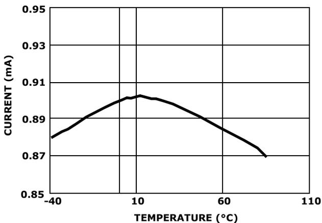
FIGURE 14. I<sub>DD</sub> CURRENT (AT V<sub>DD</sub> = 80V)
