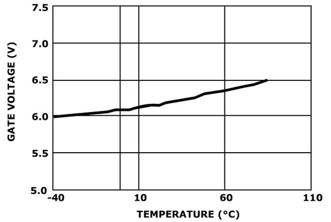
FIGURE 17. GATE VOLTAGE (AT  $V_{DD} = 10V$ )
