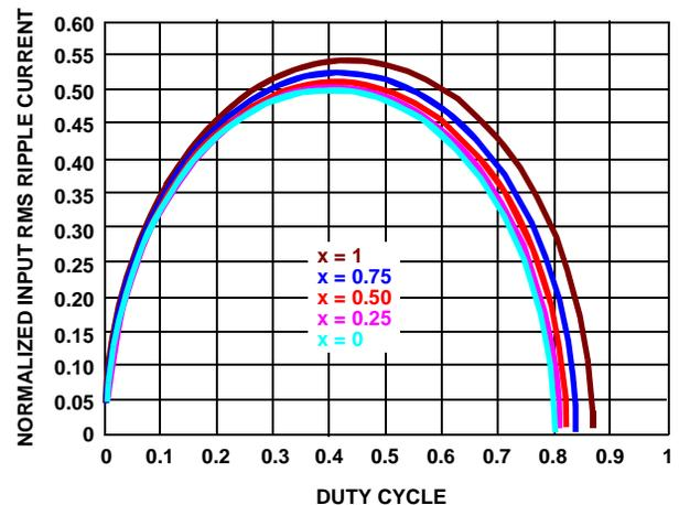
FIGURE 7. NORMALIZED RMS INPUT CURRENT FOR  $x = 0.8$
