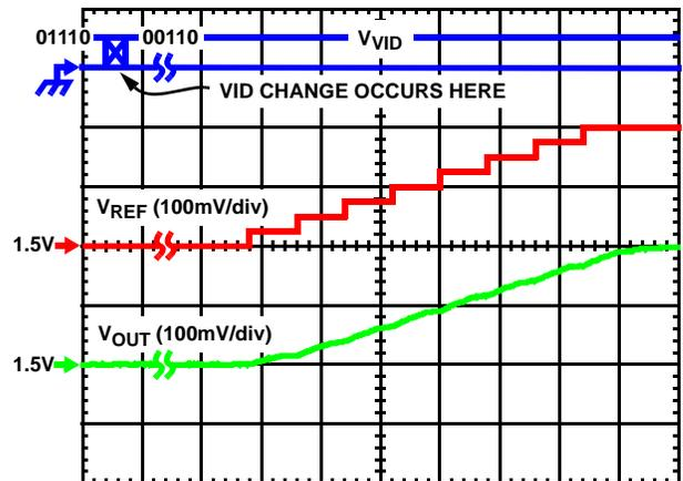
FIGURE 5. TYPICAL DYNAMIC-VID OPERATION, VRM9 DAC SETTING
