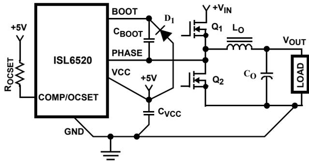
FIGURE 4. PRINTED CIRCUIT BOARD SMALL SIGNAL LAYOUT GUIDELINES
