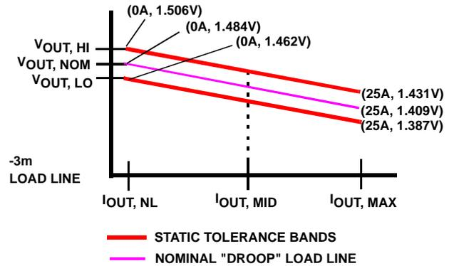
FIGURE 11. IMVP-IV™ ACTIVE MODE STATIC LOAD LINE
