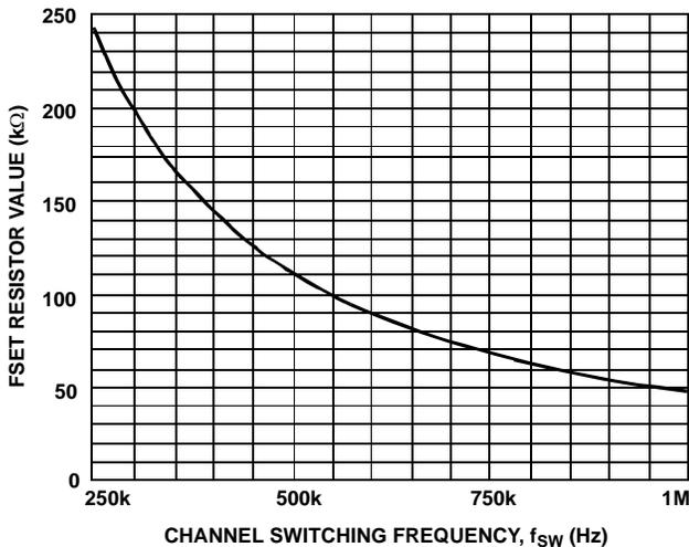
FIGURE 3. CHANNEL SWITCHING FREQUENCY vs R<sub>FSET</sub>
