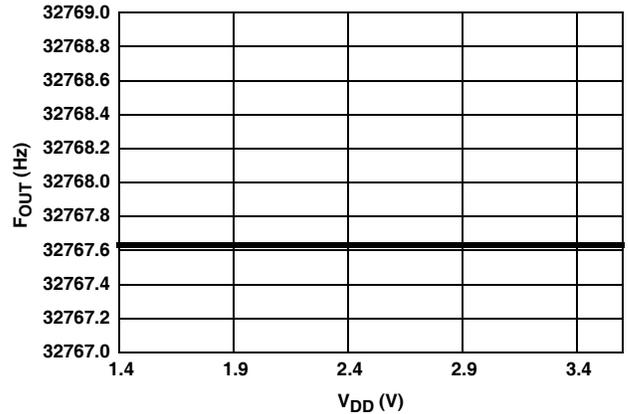
FIGURE 5. F<sub>OUT</sub> vs V<sub>DD</sub> WITH A TYPICAL 32.768KHZ CRYSTAL
