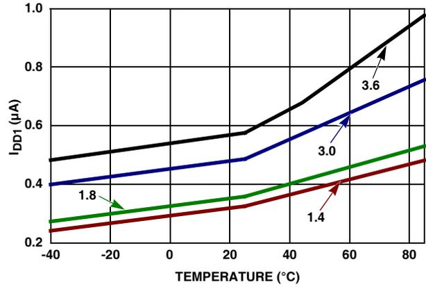
FIGURE 3. I<sub>DD1</sub> vs TEMPERATURE
