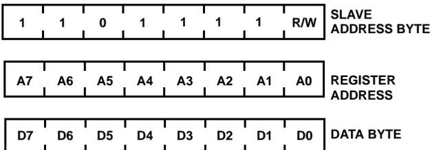
FIGURE 10. SLAVE ADDRESS, WORD ADDRESS, AND DATA BYTES
