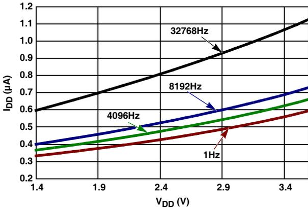
FIGURE 4. I<sub>DD</sub> vs V<sub>DD</sub> vs F<sub>OUT</sub>
