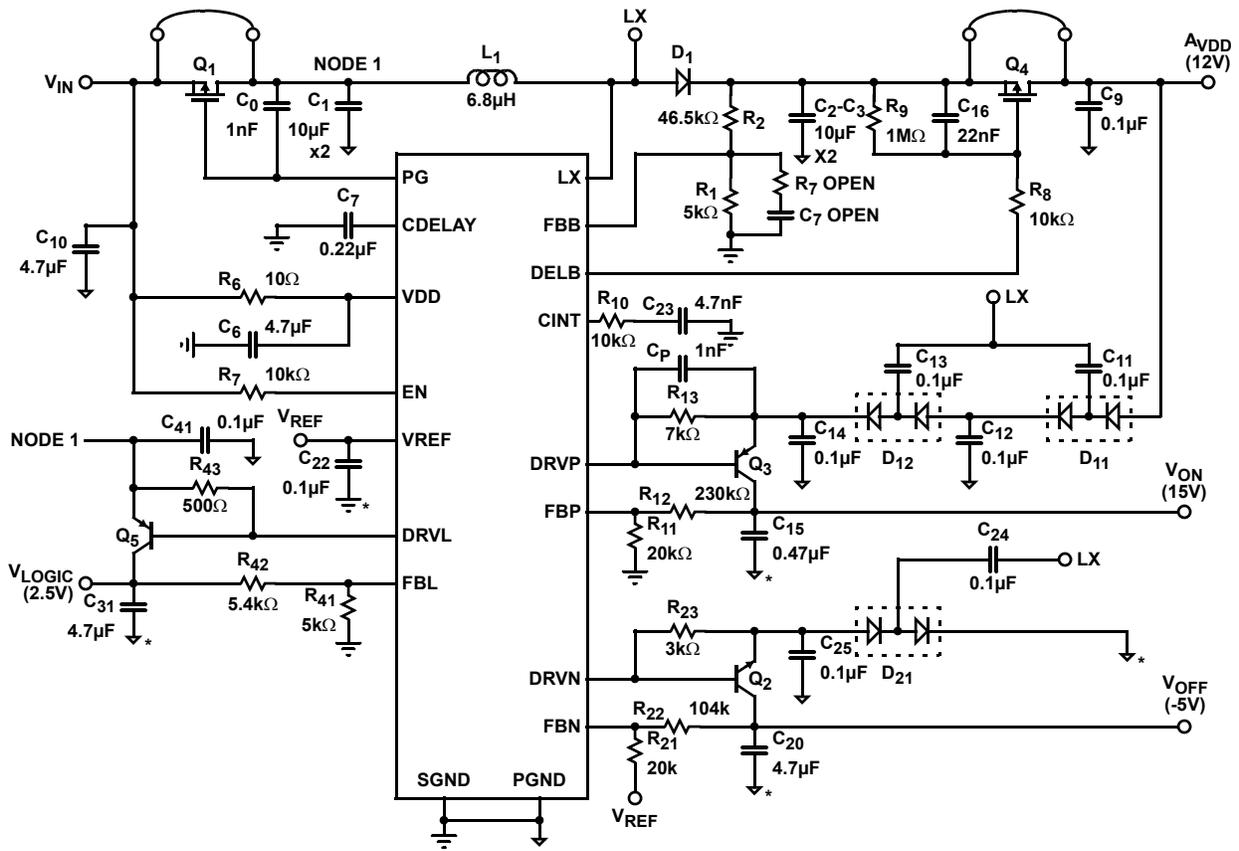
NOTE: SGND should be connected to PGND at one point only.
