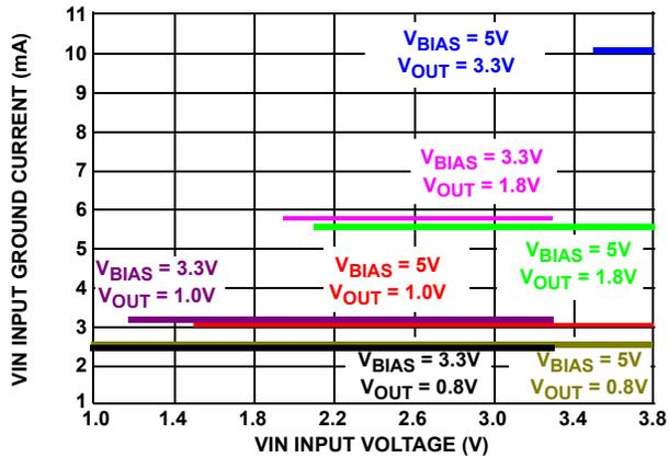
FIGURE 13. INPUT GROUND CURRENT vs  $V_{\text{IN}}$  and  $V_{\text{OUT}}$
