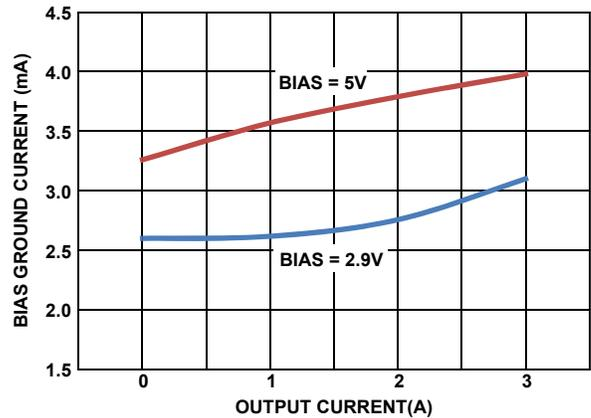
FIGURE 12. BIAS GROUND CURRENT vs LOAD CURRENT
