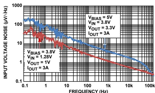
FIGURE 36. INPUT VOLTAGE NOISE vs BIAS VOLTAGE
