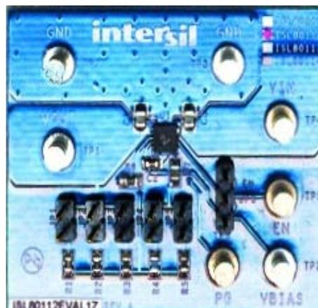
FIGURE 39. ISL80113EVAL1Z (TOP PCB LEFT, PHOTOGRAPH RIGHT)
