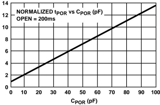
FIGURE 3. ADJUSTING t<sub>POR</sub> WITH A CAPACITOR
