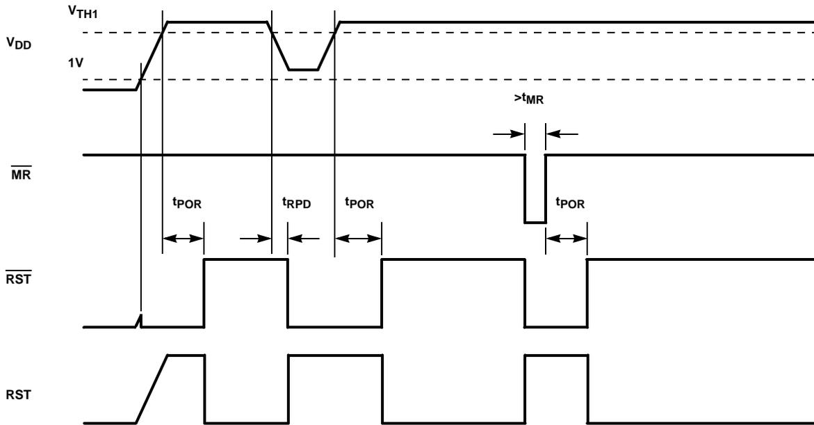
FIGURE 1. POWER-SUPPLY MONITORING TIMING DIAGRAM (WDI TRI-STATED)
